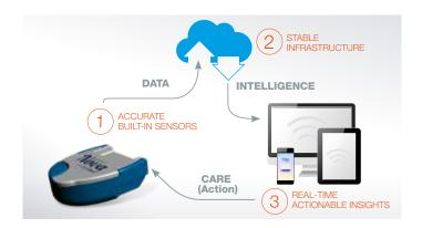
ABENA Nova uses a unique wireless connection to digital sensors to deliver actionable insights to caregivers. The sensors in the continence product continuously register changes in wetness levels and share real-time information to caregivers on a mobile device via the WetSens Monitor app.
